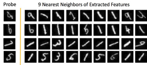
Figure 8. Feature Space Visualization. Nearest neighbors of probe images (left column). Feature representation encodes digit angle, not digit label.
